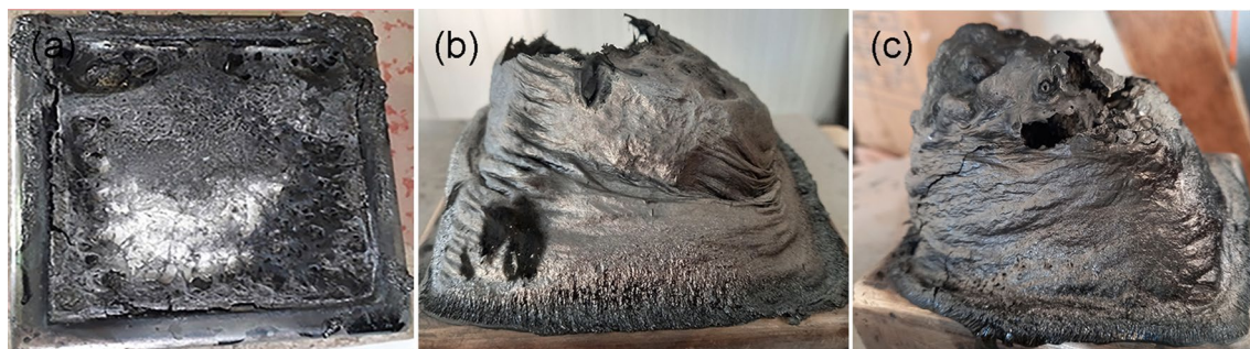
Fig. 5 Photos of char residue of TPU/IFR composites after cone calorimeter test
