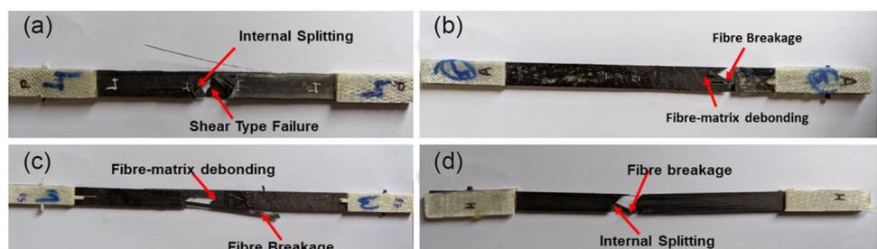
such phenomenon was a degradation of the fibre-matrix interphase. As the ageing period increased, delamination became more intense, leading to the catastrophic failure of the CFRP specimens.
