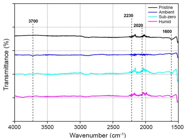
**Fig. 2** FTIR spectra of pristine and carbon/epoxy composite specimens aged under different conditions
