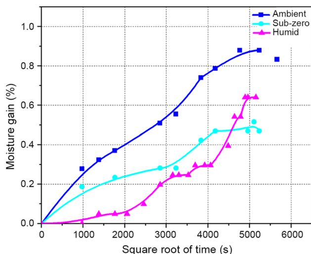
**Fig. 1** Moisture absorption curves for carbon/epoxy composite specimens aged under different conditions
