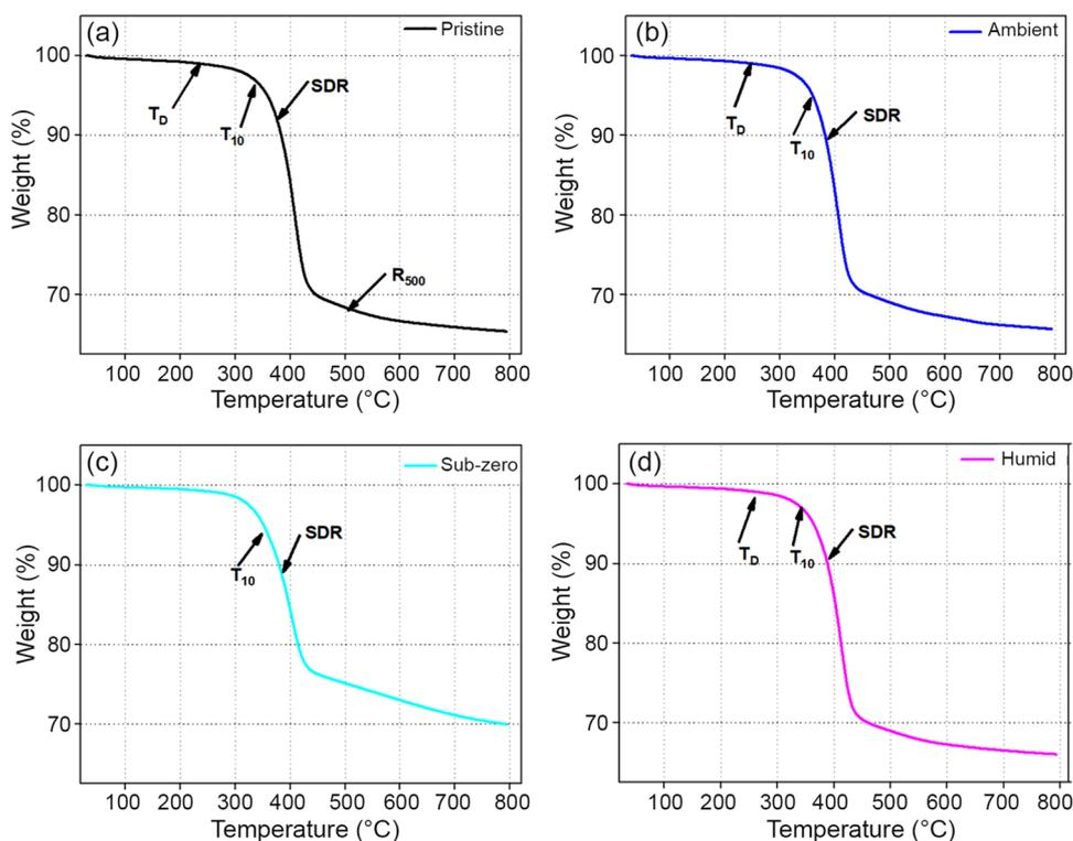
For ambient conditioned composite specimen shown in Fig. 7b, the 2% weight loss was observed at a temperature of around 249 °C. The increment was due to the water molecule entering the matrix material, which changed the chemical composition of epoxy. The 10% weight loss was observed at around 378 °C, and the rapid degradation started at around 392 °C.
