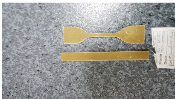
Fig. 2 Shape of mechanical test specimens of thermocompressed composites
