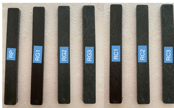
Fig. 1 Injection molded samples of graphene and MWCNT nanofillers with rectangular cross-section
