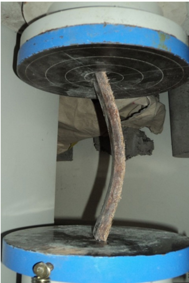
Fig. 5 Test specimen under buckling
