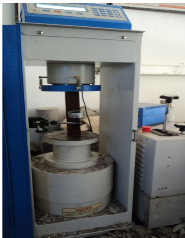
Fig. 4 Buckling test setup
