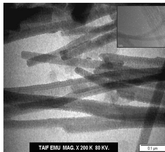
Fig. 1 TEM image of SWCNTs/PMMA composite film at concentration of 2.0 wt%, the inset shows higher resolution TEM image of SWCNTs
