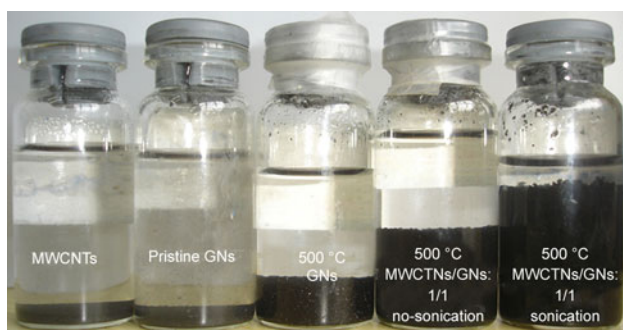
Fig. 5 States of MWCNTs, pristine GNs, GNs treated by thermal expansion, and mixtures of GN sand MWCNTs with and without ultra-sonication, in high-purity chloroform
