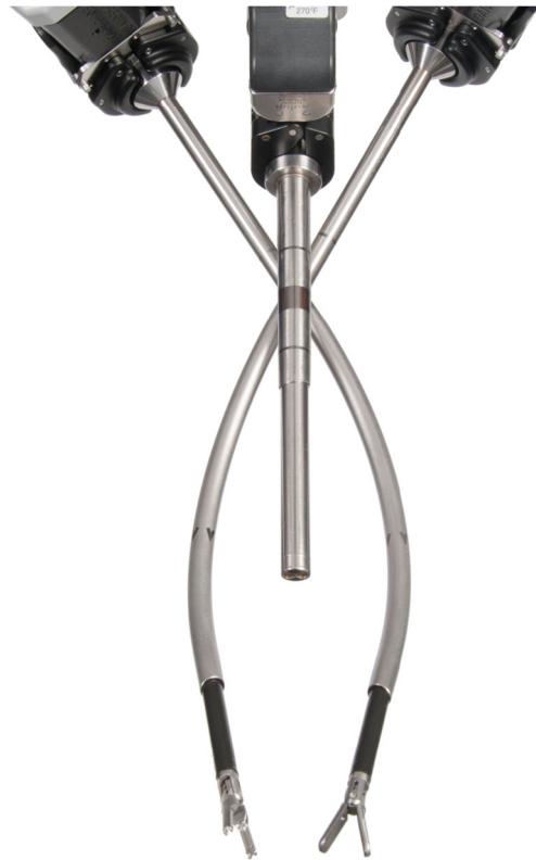
Fig. 1 The single-site robotic Da Vinci system which is a modification of the traditional system. ©[2016] Intuitive Surgical, Inc.
