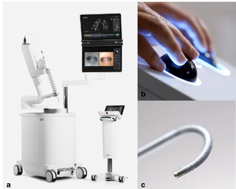
Fig. 1 a The Ion™ system (Intuitive Surgical) includes the system cart with monitor and the controller (b) that works similar to a computer mouse and roller. c The robotic catheter with a vision probe allows visualization during navigation of the airways. Images provided by Intuitive
