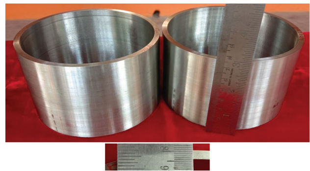
Fig. 3 Photograph of 2209 DSS cylindrical components (after machining)
