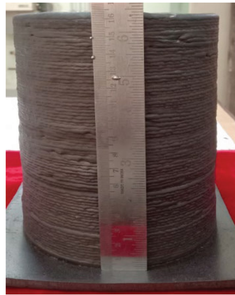
Fig. 2 Photograph of the WAAM 2209 DSS straight cylindrical component
