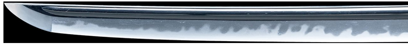
Fig. 8 Japanese sword with a hamon pattern [20]. Reprinted from [20] under CC0 1.0 license at The Metropolitan Museum of Art
