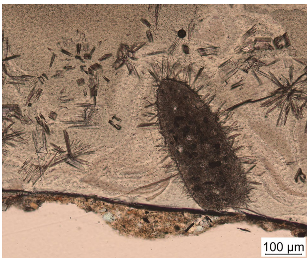
Fig. 6 Clay fragment in the glaze layer of sample A45170048_11. The glaze has changing chemistry around the clay fragment. Skeletal crystals form around the fragment, seemingly growing from the surface of the fragment into the still molten glaze
