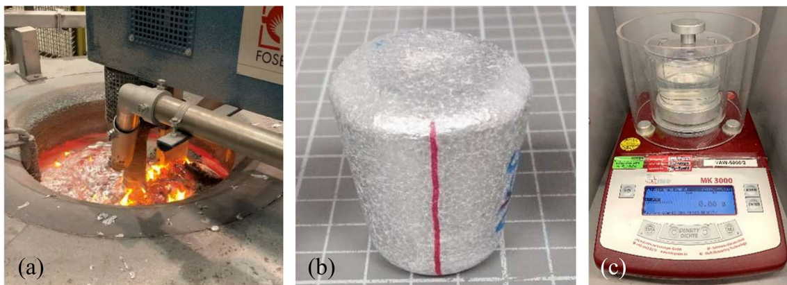
Fig. 2 (a) Preparation of the melt, (b) the RPT specimen (the red line indicates the location of the longitudinal section to be polished), and (c) the MK3000 density meter
