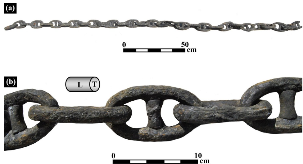
Fig. 2 The chain segment after removal of the concretion: (a) general view of the chain; and (b) the links with stud at their center
