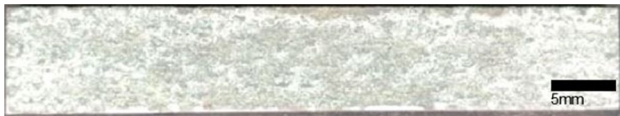
Fig. 4 Image of Al 7075-T651 unwelded base plate exposed for 48 h in EXCO solution
