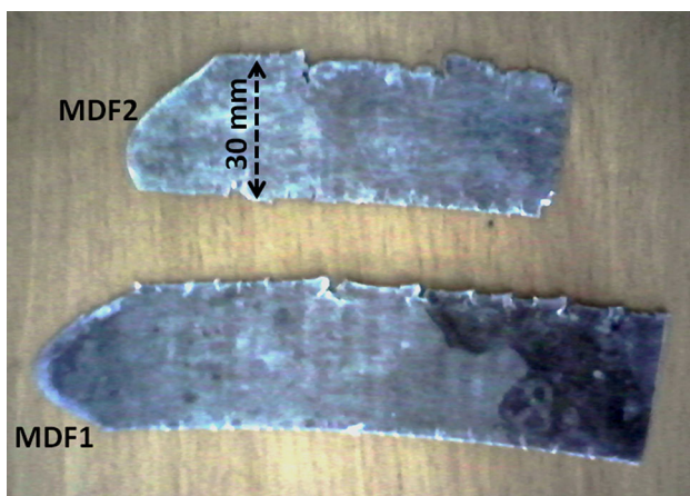
Fig. 3 Photograph of UFG alloy sheets obtained through MDF1 and MDF2 routes
