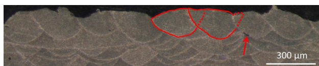
Fig. 4 Close up of track segments, showing the dimensions of the half-cylindrical melt pools. Early formation of a defect can be seen marked by the arrow
