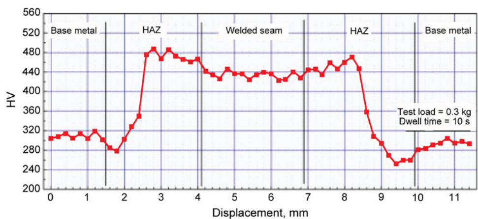
Fig. 22 Microhardness profile across 1.6 mm (0.06 in.) Q&P 980 metal-active-gas-welded joint. HAZ heat-affected zone
