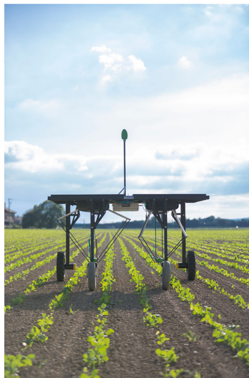
Fig. 1 Technological development is a key driver of change in soil management. The example is one of the first agricultural robots being close to commercialization, which are small and lightweight, so that they can reduce weight and contact stresses and facilitate smaller-scaled field patterns. As its main task, this robot can make weed control much more efficient. It identifies the weeds with a sensor and sprays each plant individually. The developers are also working on an implement for organic farming. (photo credits: Ecorobotix autonomous robot weeder, 2016)
