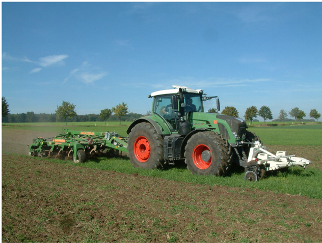
Fig. 4 In front of the tractor, a sensor detects soil texture via the conductivity. Sandy soil with low conductivity is being tilled at a deeper working depth than a clayey soil with high conductivity. Data acquisition and implementation are done in real time. (photo credits: Hans-Heinrich Voßhenrich)
