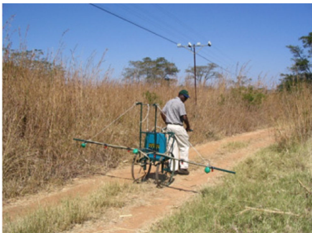
Fig. 5 A hand-pulled six-nozzle sprayer for herbicide application. This equipment is relatively inexpensive and allows for faster application. Photo credit: Christian Thierfelder, CIMMYT
