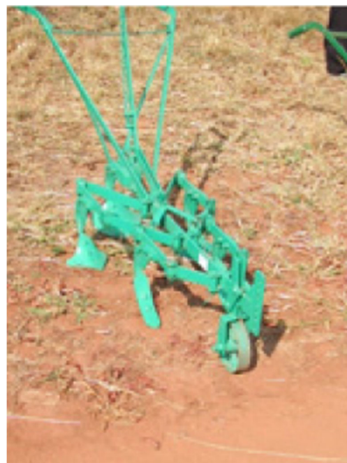
Fig. 2 The animal drawn cultivator is commonly used by smallholder farmers with access to animal draft power. These cultivators superficially disturb the soil, while still providing some of the weed suppressing benefits associated with tillage practices. Such cultivators can provide labor relief to smallholder farmers. Photo credit: Joseph Kienzie, FAO
