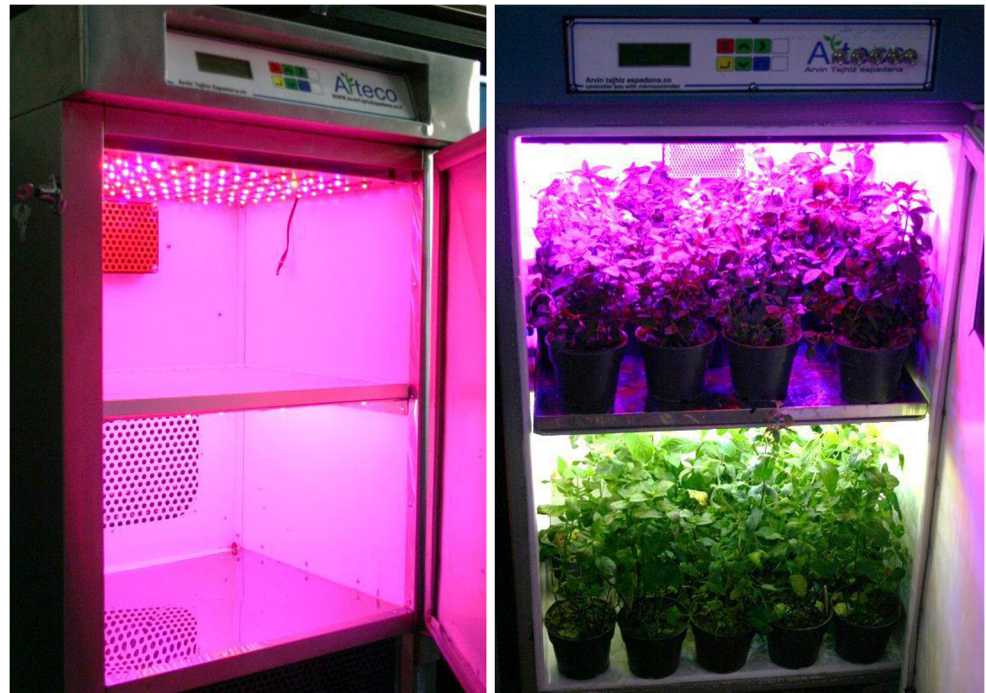
Fig. 1 Constructed light emitting diode (LED) incubator with mint plants grown under irradiation platform. This growth chamber is in size of 1.0 width×0.6 depth×1.5 m height, equipped with microcontroller for setting the plant growth parameters of light, temperature and humidity to support plant superior growth
