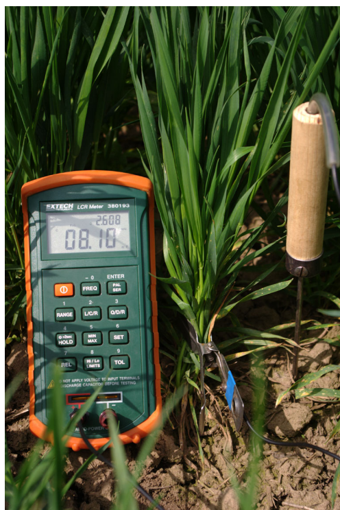
Fig. 1 Measurement of cereal root system size on the basis of its electrical capacitance
