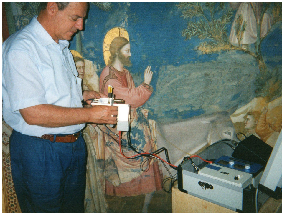
Fig. 9 EDXRF device for elemental analysis of frescos in the Chapel of the Scrovegni, painted by Giotto in Padua between 1303 and 1305. Two measuring heads were employed: one composed of a Hamamatsu X-ray tube working at 10 kV and 1 mA, and a Si-PIN detector, for the analysis of sulfur; the second composed of an Oxford X-ray tube with Mo-anode, for analysis of medium-high Z elements, is composed of a mini X-ray tube working at 30 kV and 500 \mu A and a Si-PIN detector
