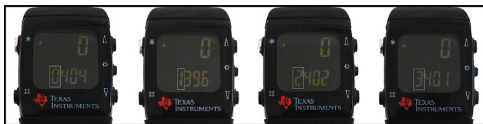
Fig. 3. CHRONACT systems displaying the classification results of 0 (LOW-STA), 1 (LOW-ACT), 2 (MED) and 3 (HIGH). Additionally, the devices show memory consumption (top right) and debug information for radio communication (bottom right).
