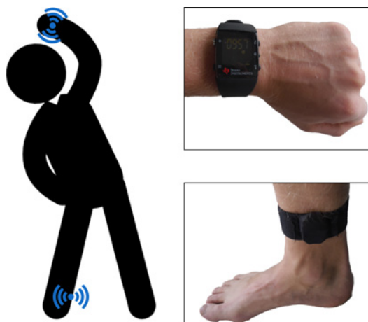
Fig. 1. Sensor positions on the left wrist and right ankle and the two components of the CHRONACT system.
