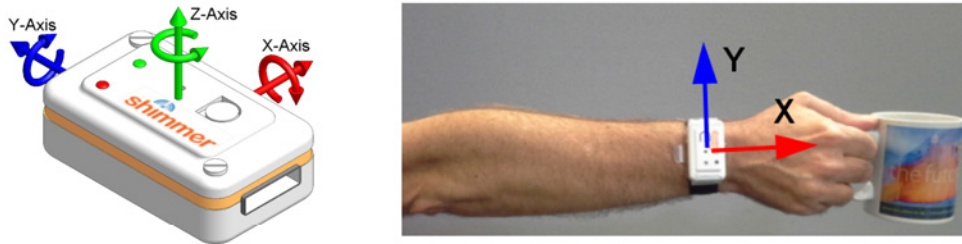
Fig. 1. Sensor module showing the coordinate system for the positive direction of the accelerometer axes and rotation for the gyroscope (left); when worn on the wrist showing the X and Y axis, the Z axis points away from the plane (right).
