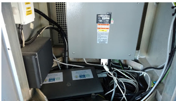
Fig. 7 The computer for data registration connected to the Furuno radar with ARPA
