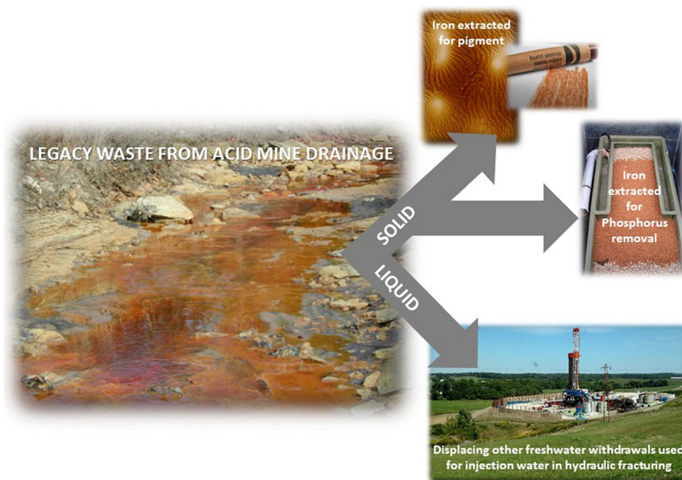
Fig. 1 Conceptual diagram of waste from coal mining (acid mine drainage) repurposed to meet resource demands within the energy industry (injection water for hydraulic fracturing) and resource demands for other markets (pigment and phosphorous remediation). Image for phosphorus remediation used with permission from Kate Heal, University of Edinburgh ( www.geos.ed.ac.uk/research/cccs/water.html )
