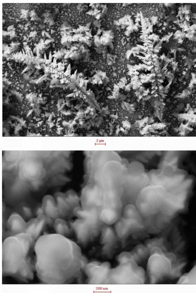
Fig. 2 FESEM images of Au/nano-Au-Hist electrode surface with different magnifications. The electrodeposition solution contained 20 \text{ mmol L}^{-1} \text{ HAuCl}_4 + 0.5 \text{ mol L}^{-1} \text{ H}_2\text{SO}_4 + 150 \text{ mmol L}^{-1} \text{ histidine} . The electrodeposition potential was 0 V, and the electrodeposition duration was 600 s
