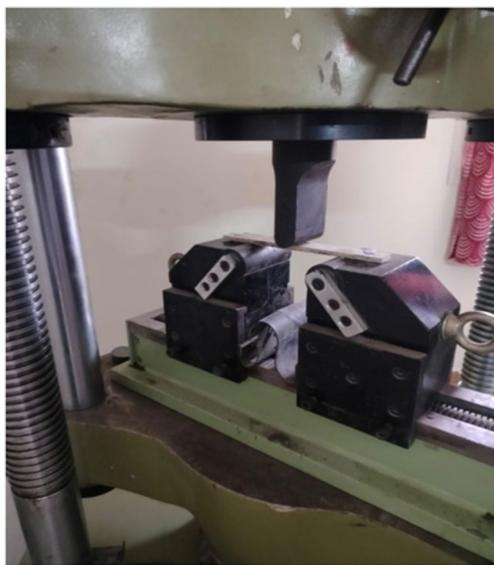
**Fig. 13** Flexural testing machine
