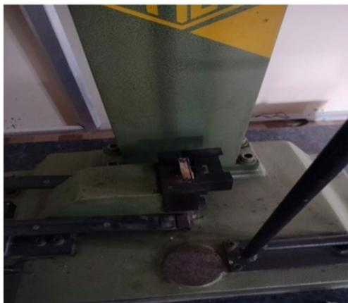
**Fig. 10** Impact testing machine
