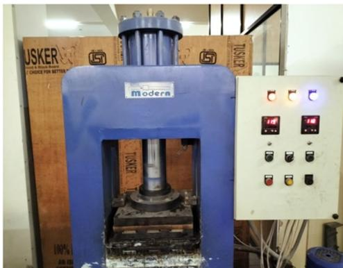
**Fig. 5** Compression moulding machine
