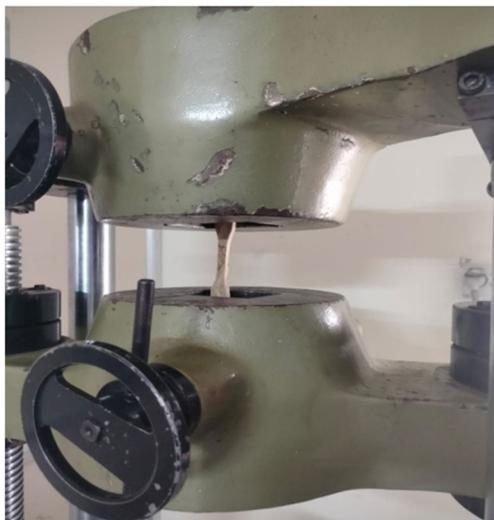
Fig. 7 Tensile testing machine
