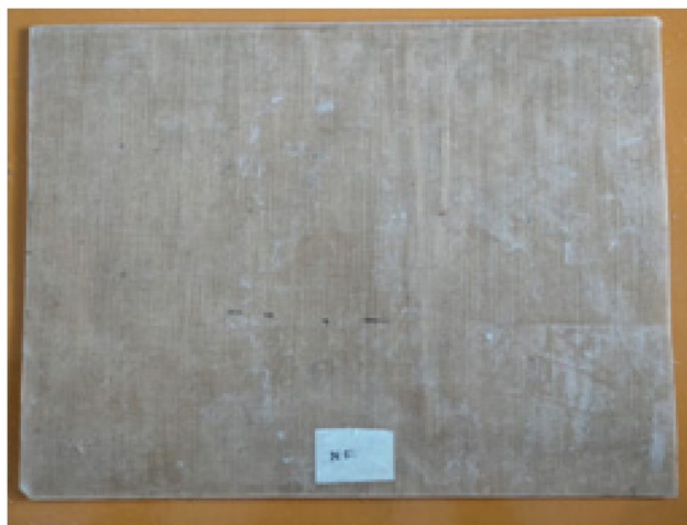
Fig. 3 Actual developed areca fiber mat composites
