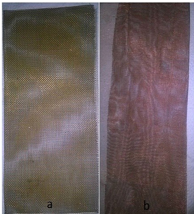
Fig. 2 Electrode materials: a brass mesh and b copper mesh
