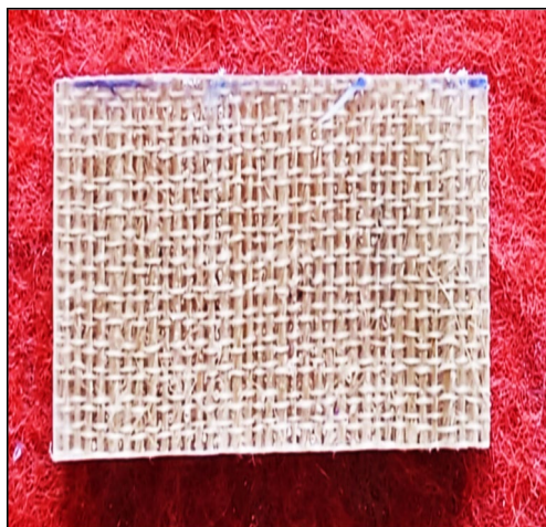
Fig. 4 Fabricated kenaf fiber and nanocellulose reinforced composite material
