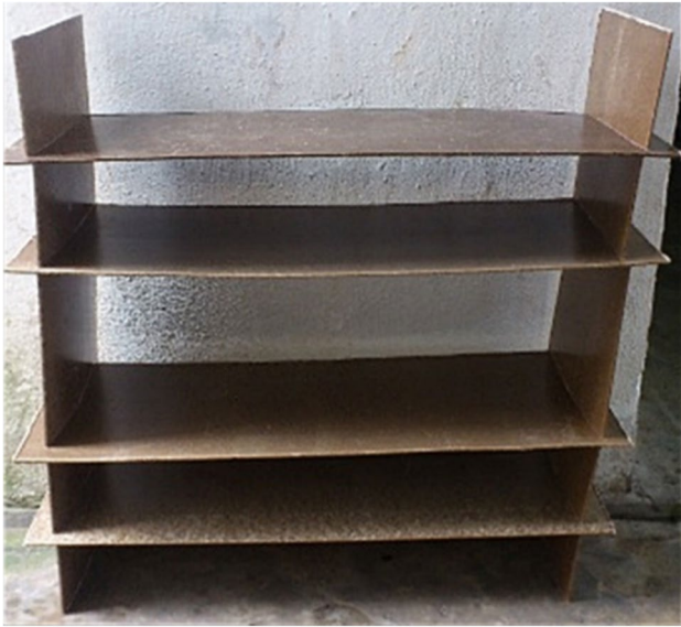
Fig. 6 Shoe rack made of kenaf fibre reinforced polymer composites. Reproduced with permission from ref. [48]. Copyright 2019 Elsevier
