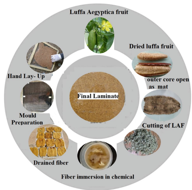
Fig. 1 Composite laminates fabricated in the present study
