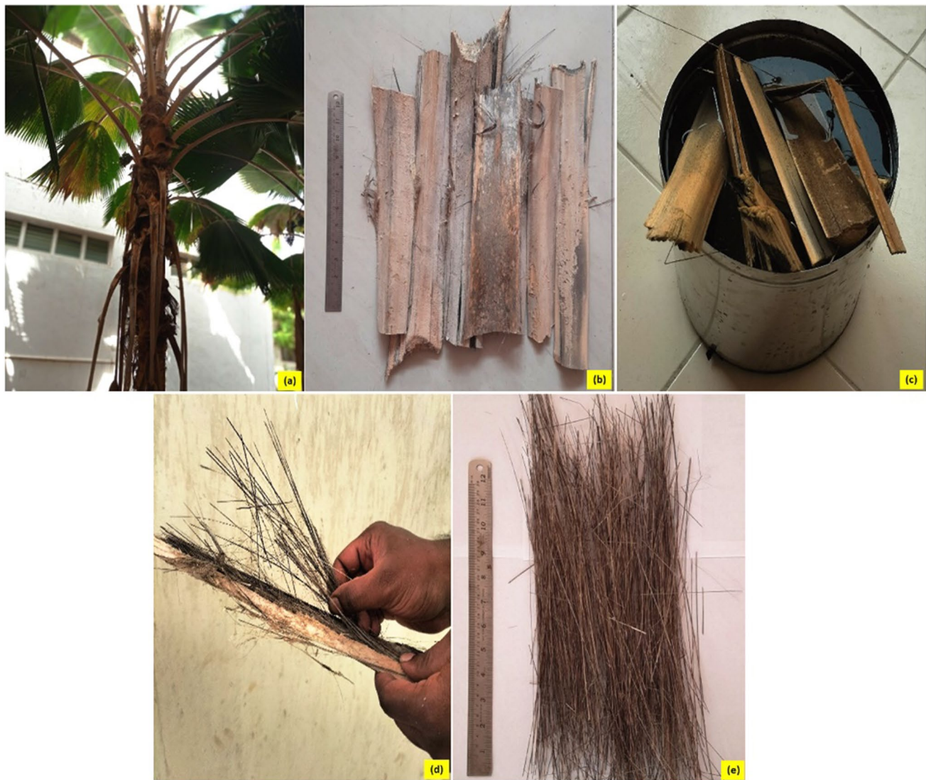
Fig. 1 Extraction of Licuala grandis tree leaf stalk fiber. a Licuala grandis tree, b collected leaf stalks of Licuala grandis tree, c soaking of leaf stalk, d fiber extraction, and e extracted Licuala grandis tree leaf stalk fibers
