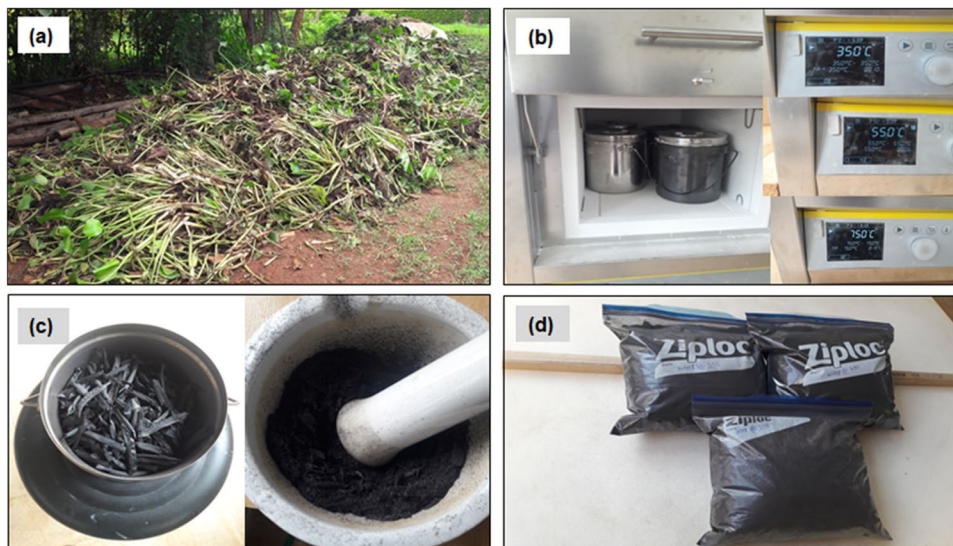
Fig. 1 Steps of biochar production from water hyacinth. a Water hyacinth collected from Lake Tana. b Water hyacinth pyrolysis in different temperatures in an electric furnace. c Biochar produced from water hyacinth and crushing. d Biochar stored for analysis after sieving
