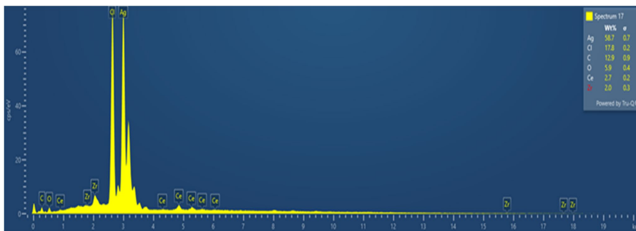
Fig. 6 EDX analysis of Tridax procumbens -mediated Ag-Fu NPs with various elemental compositions
