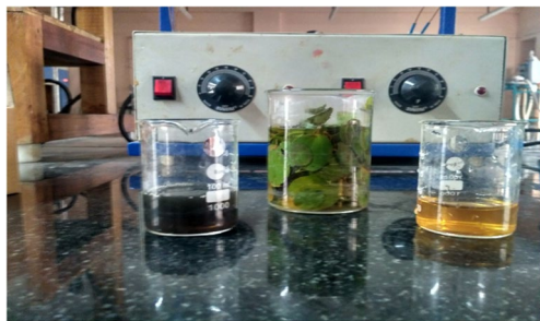
Fig. 1 Visual observations for the formation of iron nanoparticles (a reaction mixture (a) before reaction, b) after reaction)
