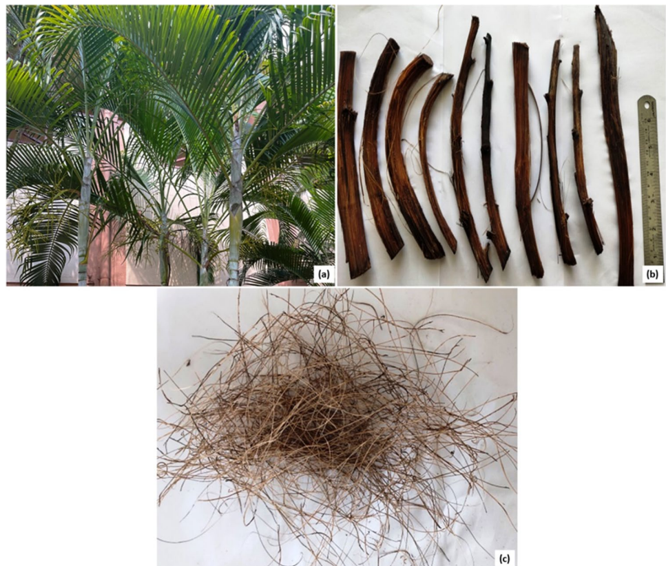
Fig. 1 Extraction of Dyopsis lutescens peduncle fiber: a Dyopsis lutescens tree, b collected peduncles of Dyopsis lutescens , and c extracted Dyopsis lutescens peduncle fibers
