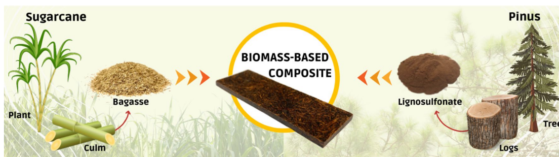
Fig. 2 Biomass-based composite: sugarcane bagasse fibers as a reinforcement of lignosulfonate-based phenolic matrix
