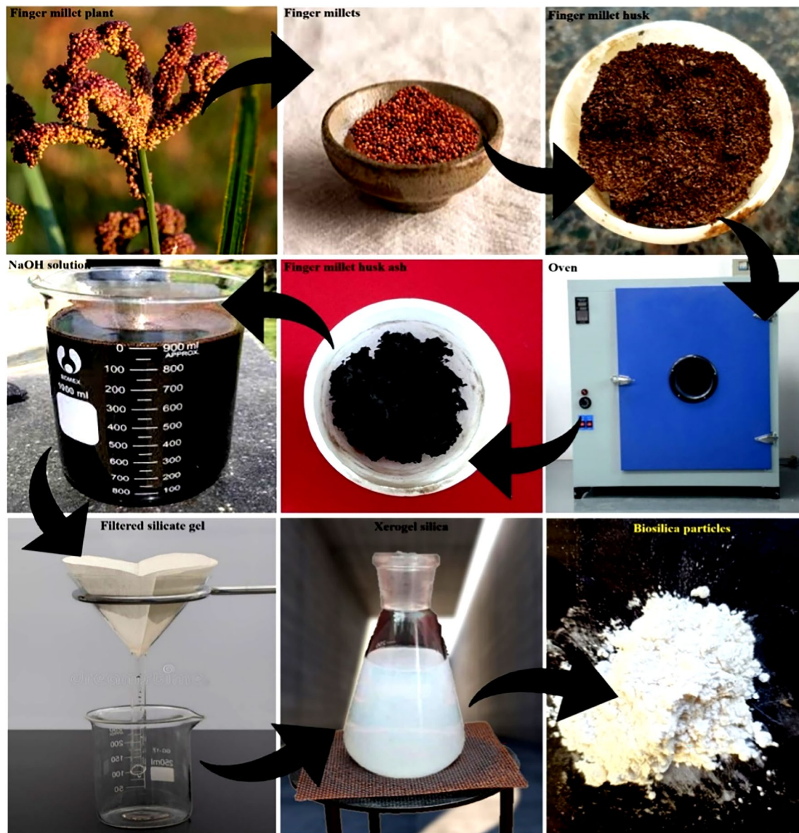
Fig. 3 Biosilica preparation route from finger millet husk
