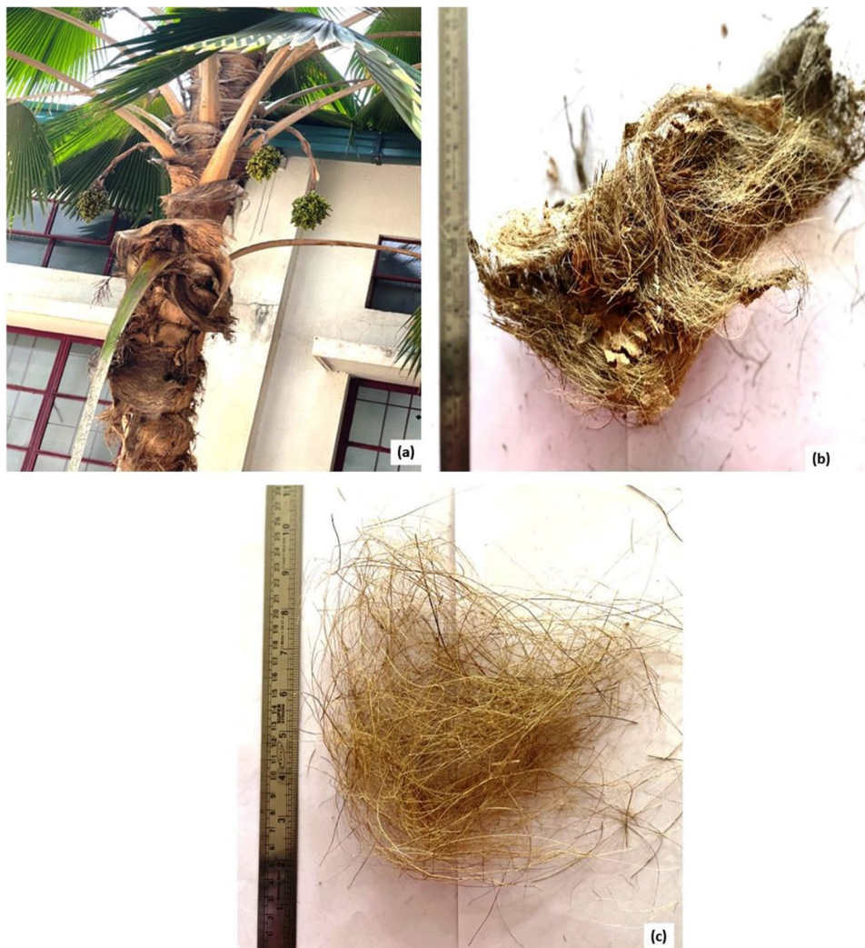
Fig. 1 Extraction of Licuala grandis leaf sheath fiber (a) Licuala grandis tree (b) Collected leaf sheaths of Licuala grandis and (c) Extracted Licuala grandis leaf sheath fibers
