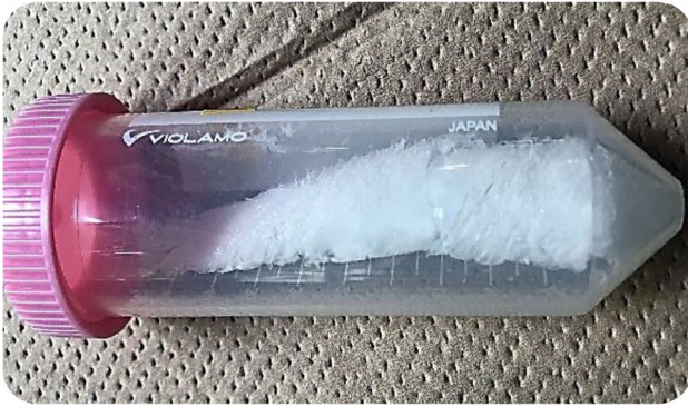
Fig. 1 Purified EPS product obtained from glycerol substrate, using Bacillus sonorensis NTV10, under thermophilic condition
