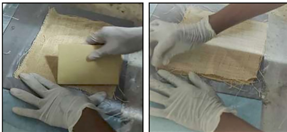
(a) Composite laminate preparation using hand lay-up technique
