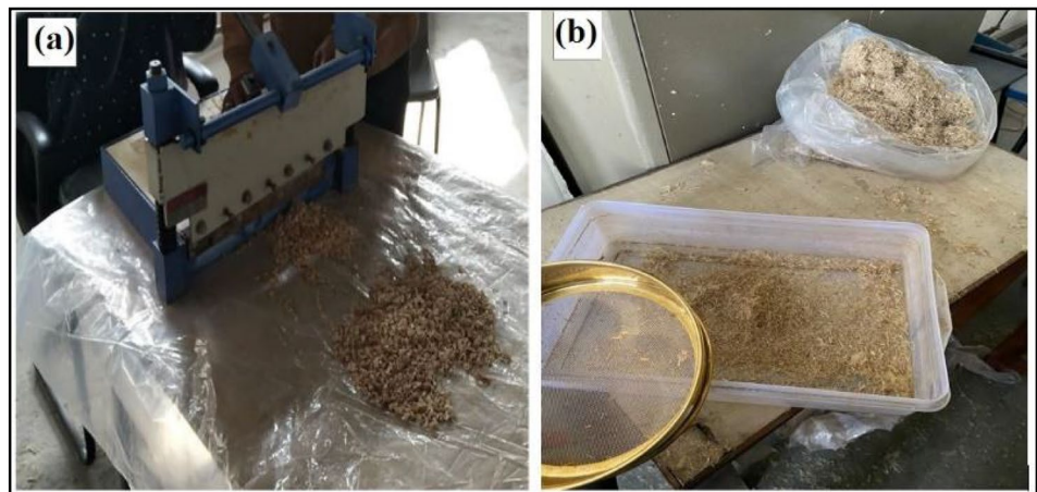
Fig. 1 Himalayacalamus falconeri fiber undergoing a chopping process and b sieving process
