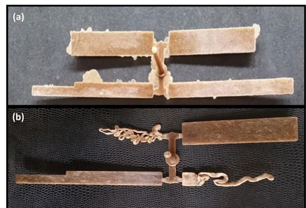
Fig. 3 Defects during direct injection molding (DIM) process, a flash and b short shot
