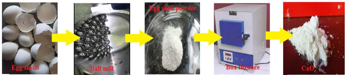
Fig. 2 Calcination process for egg shells
