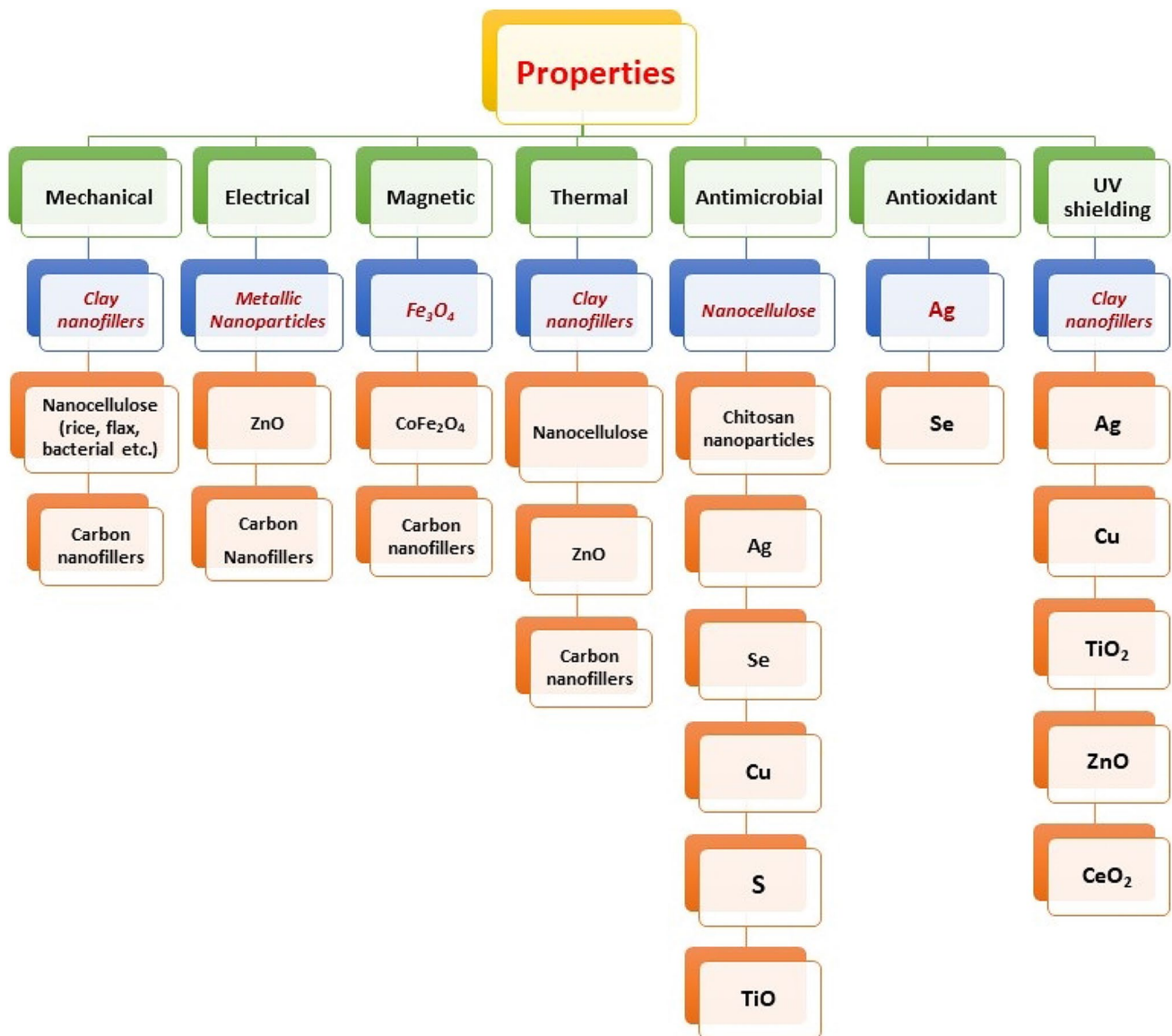
Fig. 6 Influence of nanofillers on performance of polymer composites
