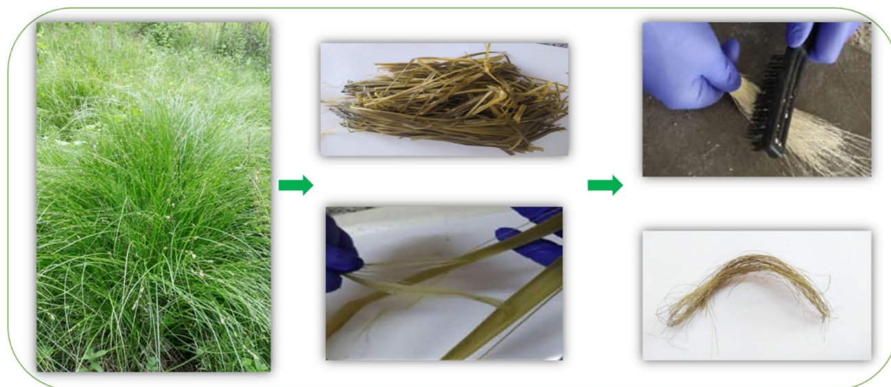
Fig. 1 The schematic diagram of the fiber extraction with the Carex panicea plant image
