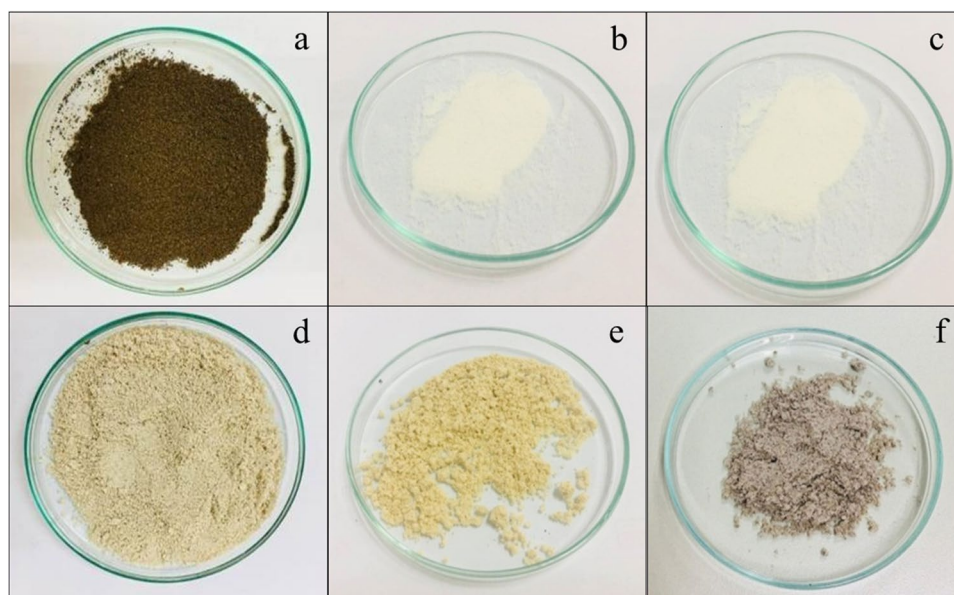
Fig. 2 SL images pretreated with alkali (a), delignification (b), and alkali-delignification (c), and KC pretreated with alkali (d), deproteinization (e), and alkali-deproteinization (f)
