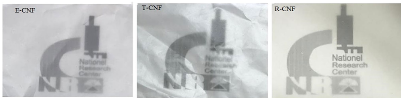
Fig. 5 Aspect of nanopapers prepared from E-CNFs, T-CNFs, and R-CNFs
